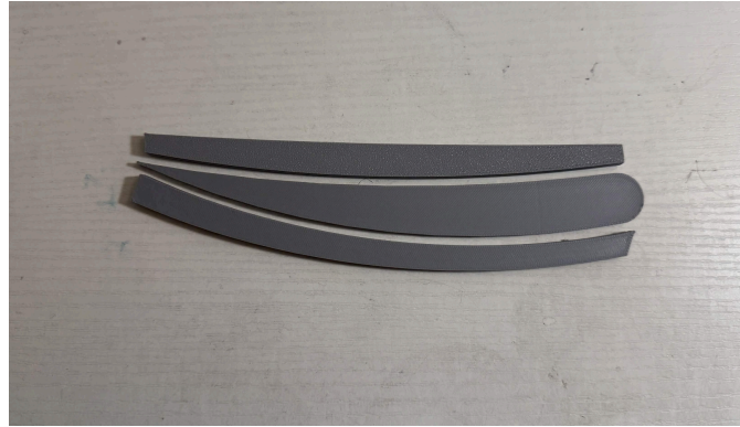
Figure 8.2. 3d printed cross section, upper and lower template used to match curvature.
