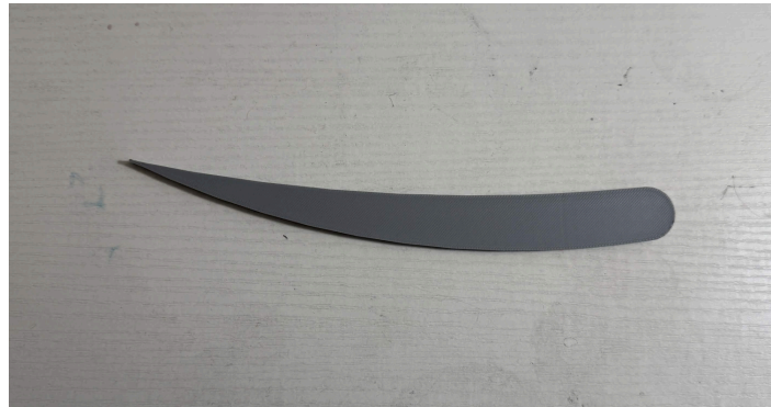
Figure 8.1. 3d printed cross section, a template used to cut and outline xps foam
