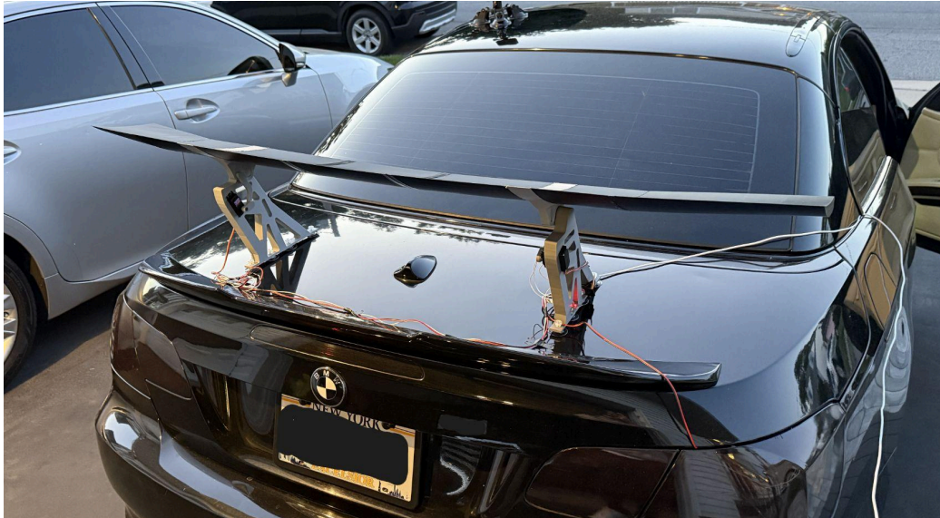
Figure 17. AVIWS mounted on BMW E33 trunk lid, rear view showing full wing assembly and bracket geometry.
