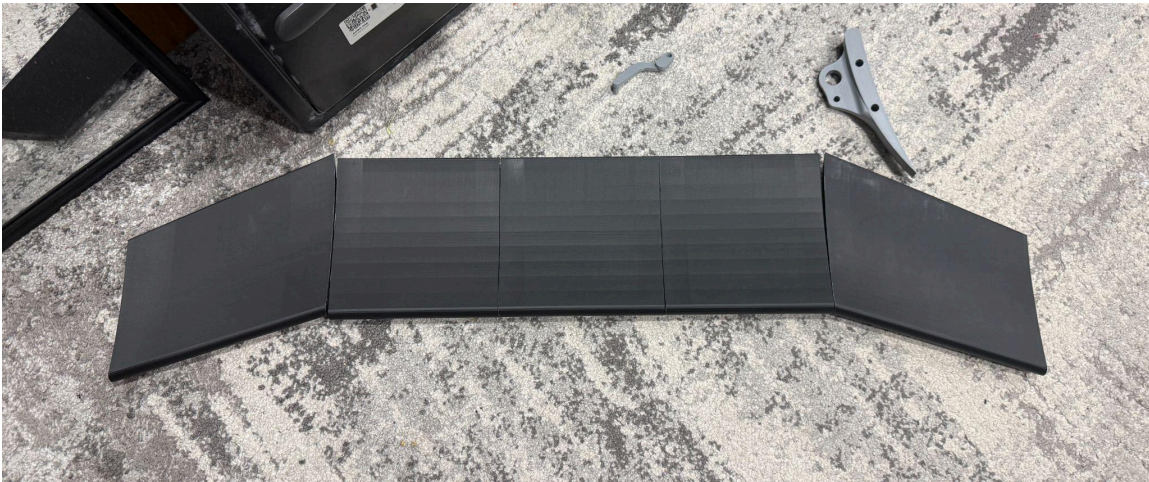
Figure 10. Assembled wing, attached via dowels. Will be plastic welded to ensure increased rigidity
