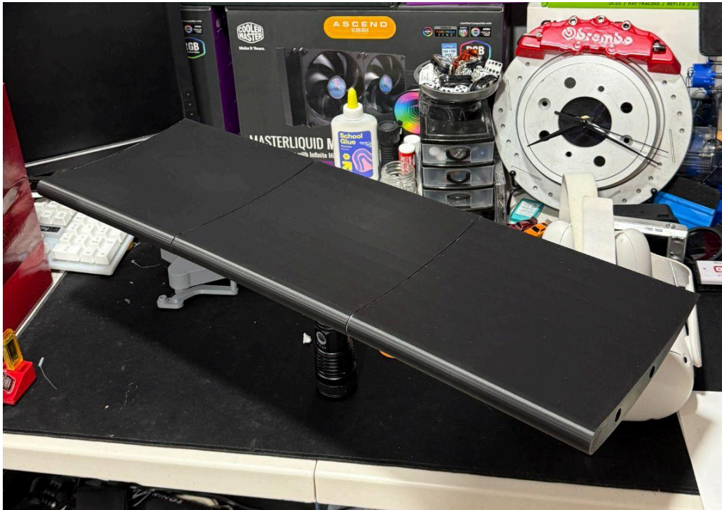
Figure 10. 3 of the 200mm wing pieces are attached via dowels, balancing on the center of mass point of the air foil.
