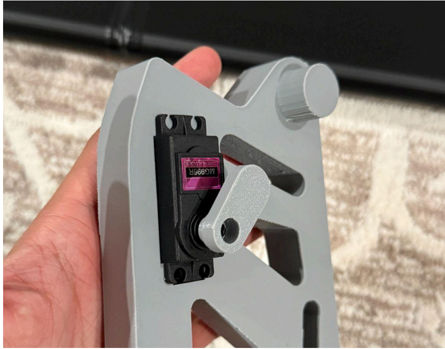
Figure 13. Custom designed servo horn to attach to the main connecting arm.
