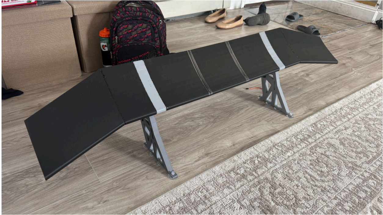
Figure 11.2 Fully assembled and welded wing element prior to mounting.
